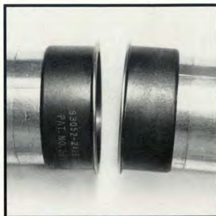
Not an Acceptable Assembly Allowance (Beyond Design Limit of 4 deg)
