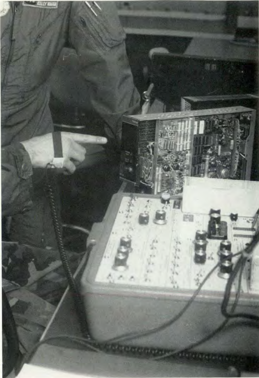
The grounding strap on this technician's hand will not only keep a big blue spark from leaping off the finger; it will also prevent unseen or unsensed voltage from damaging sensitive components.
